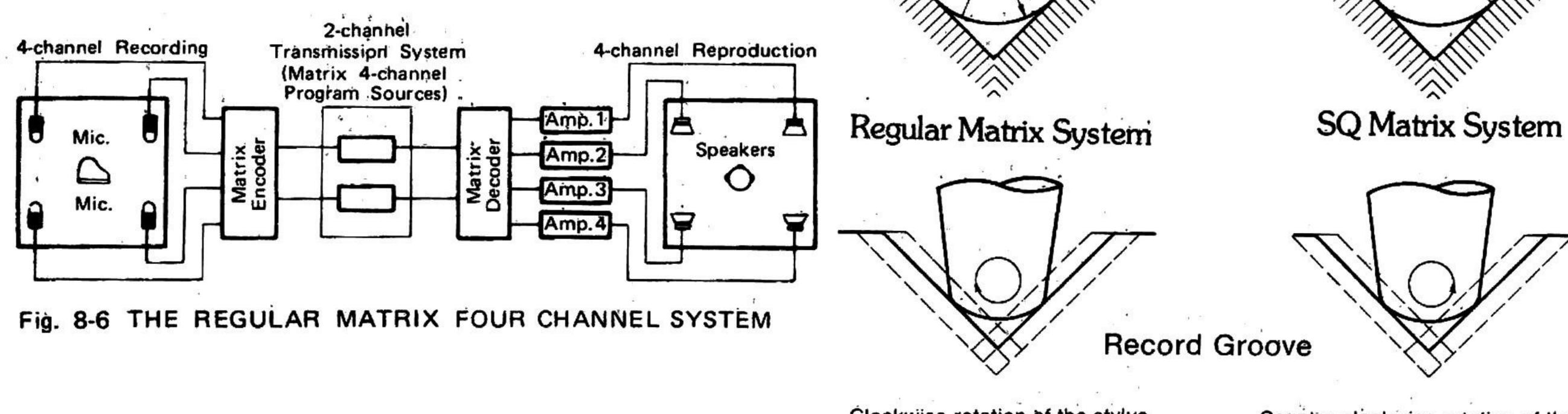
Clockwise rotation of the stylus (modulation of Left Rear signal)
