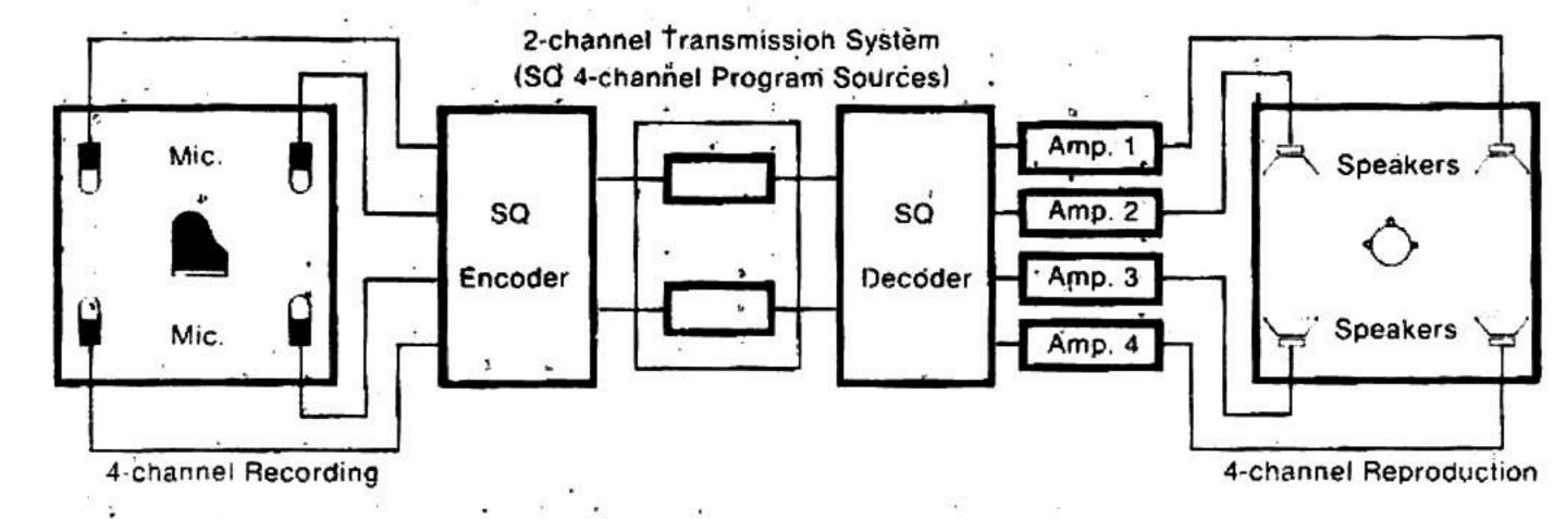
principle, by introducing an additional phase difference of 90 degrees, with the left rear channel information translated into a clockwise circular motion and the right rear channel information translated into a counter-clockwise circular motion of the stylus tip. This principle is called "circular modulation". Thus, as the record rotates, a clockwise helix is produced for the left rear channel, and a counter-clockwise helix for the right rear channel.
