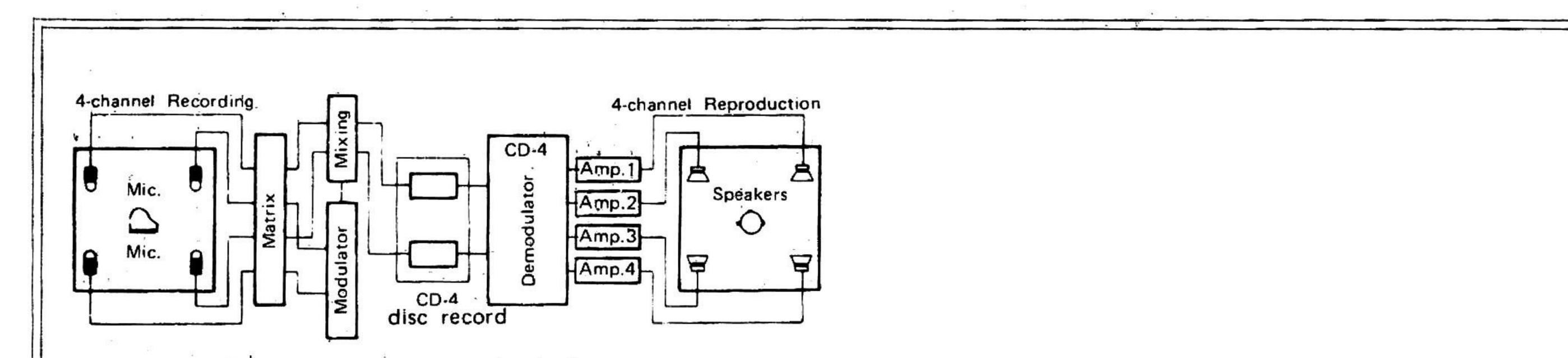
FOUR-CHANNEL DISC (CD-4 DISC) SYSTEM
