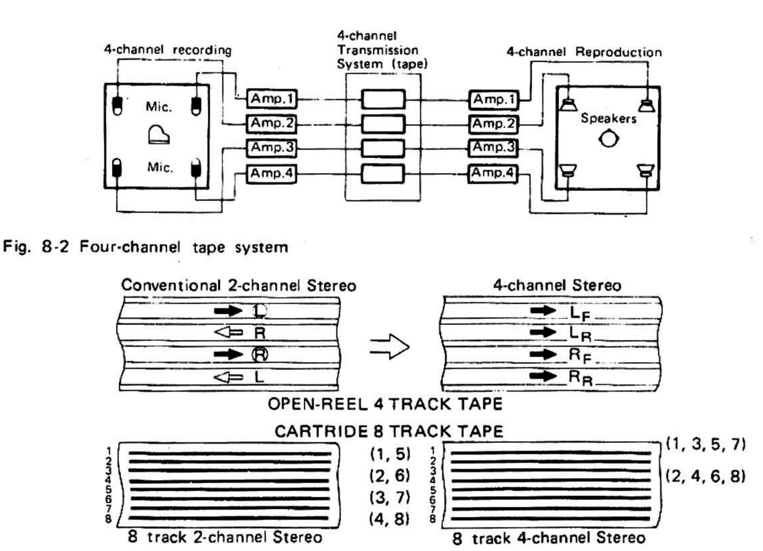
Fig. 8-3 OPEN-REEL AND CARTRIDGE FOUR-CHANNEL TAPE
